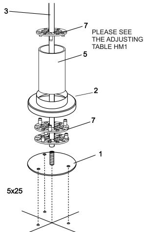
FIXING FITTINGS ON THE GROUND ARE NOT SUPPLY, THEY MUST BE CHOOSE IN FUNCTION OF FLOOR.(PLEASE TAKE PRECAUTION MEASURES IN CASE OF HEATING FLOOR).
